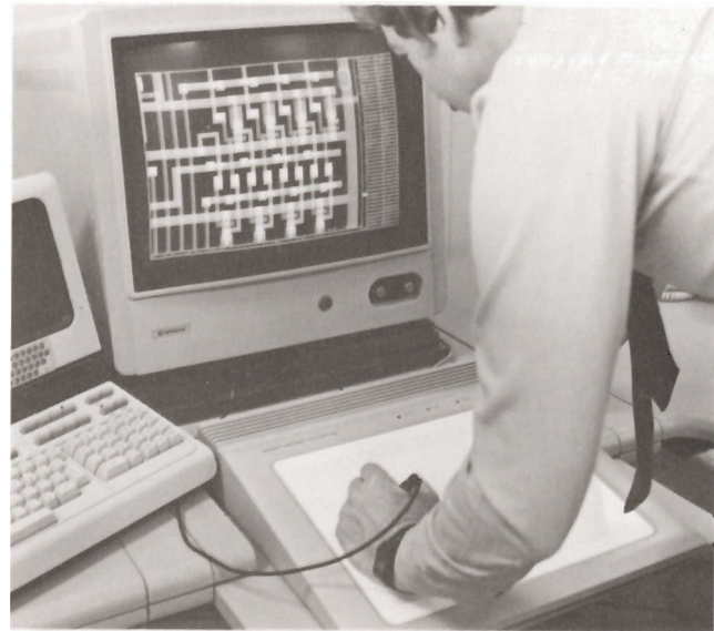
Computers are helping engineers plan, draw, check and test circuit designs. Bill McCalla, from HP Design Aids in Cupertino, uses the stylus of a graphics tablet to modify an integrated circuit design stored in the computer's memory.
