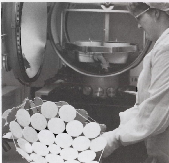
Cheryl Lohman unloads a planetary of wafers from a sputtering system that applies a thin coat of aluminum to each wafer.
